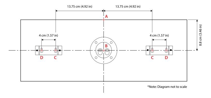
We recommend anchoring your speakers by mounting them to a stud. A stud finder can be used to easily locate them. Most homes are built with 16" (40.6 cm) on-center studs, which means there should be a stud every 16" (40.6 cm). If you have trouble finding studs on a wall, verify how far apart they are in the home by locating and measuring them on another wall. If a stud is not available, drywall anchors must be used.
