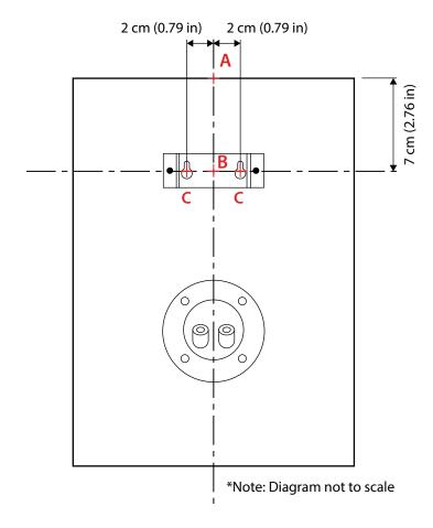
We recommend anchoring your speakers by mounting them to a stud. A stud finder can be used to easily locate them. Most homes are built with 16" (40.6 cm) on-center studs, which means there should be a stud every 16" (40.6 cm). If you have trouble finding studs on a wall, verify how far apart they are in the home by locating and measuring them on another wall. If a stud is not available, drywall anchors must be used.
