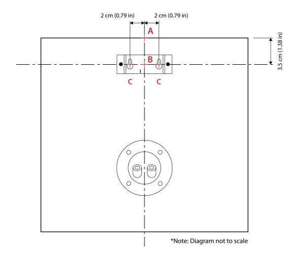
We recommend anchoring your speakers by mounting them to a stud. A stud finder can be used to easily locate them. Most homes are built with 16" (40.6 cm) on-center studs, which means there should be a stud every 16" (40.6 cm). If you have trouble finding studs on a wall, verify how far apart they are in the home by locating and measuring them on another wall. If a stud is not available, drywall anchors must be used.
