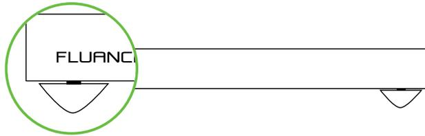
1. Use the bubble level to check the position of the base and rotate the 4 feet as shown below to confirm the base is level.
