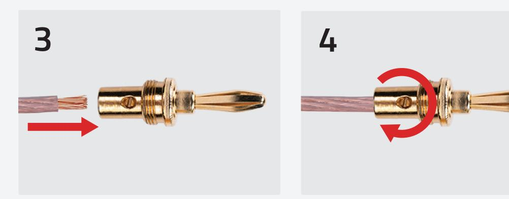
Loosen the screws on the Plug and insert 1/2 inch of stripped wire into the Plug. Firmly tighten the screws onto the wire.
