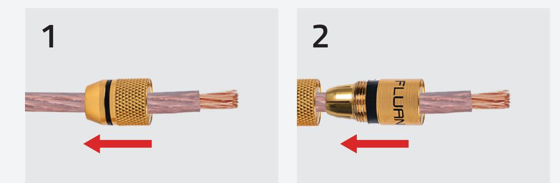
Remove the Collar from the Sleeve and install on speaker wire. Loosen and remove the Plug from the Sleeve and install the Sleeve onto the speaker wire.
